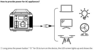
② Long press the AC control switch button for 3S, the AC indicator on the screen will light up, then connect he power cord of the electrical appliance to the AC power socket, this power station start to power your
