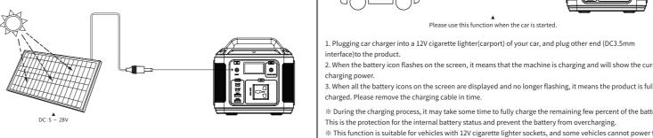
1. Place the solar panel toward the sunlight, then connect the power station to the solar panel with the DC35135mm interface cable for charging. 2. When the battery icon flashes on the screen, it means that the machine is charging and will display the
